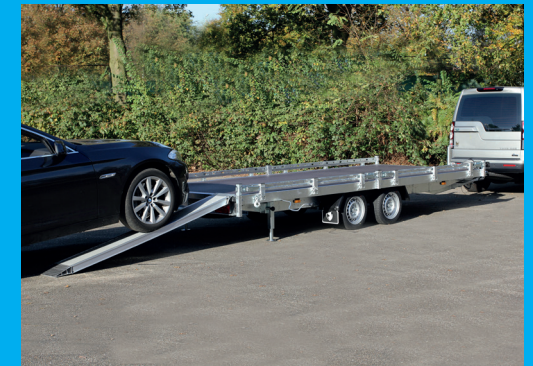
Standard: available in 2700, 3000 or 3500 kg. Max. Gross Weight (3500 kg also as a 3-axle trailer).
