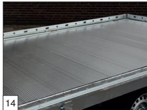
Option: floor of aluminium profiles instead of plywood floor.
