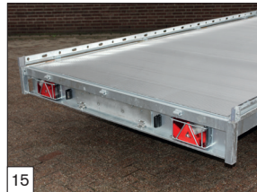
Option: an aluminium profil floor and light protection at the rear.
