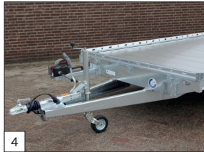
Standard: a bolted V-drawbar and a heavy duty jockey wheel assembled.
