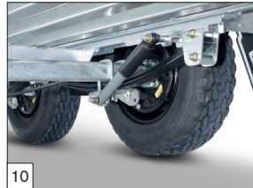
Option: parabolic axles incl. shock absorbers are possible for all Indigo HF models in 3500kg. Tyres 195/50 R13 are with black rims.
