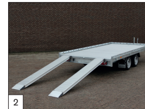
Standard: available in 2700, 3000 or 3500 kg. Max. Gross Weight (3500 kg also as a 3-axle trailer).
